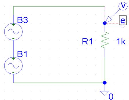
Use two VSIN sources, one R resistor, one GND-ANALOG analog ground and one MARKERS / MARK VOLTAGE voltage probe. Generate the DC component A0 as an DC option of B1.
